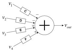
Figure 12. Block diagram of summer
