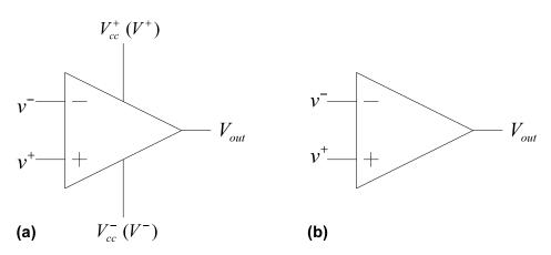
Figure 1. Op amp symbols: (a) with explicit power supplies, (b) simplified
