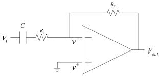
Figure 15. High-pass filter
