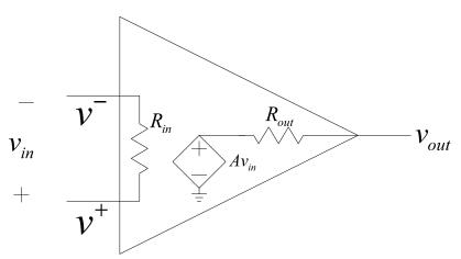
The input is:  $v_{in} = v^+ - v^-$ . The output is:  $v_{out} = Av_{in} = A(v^+ - v^-)$ .
