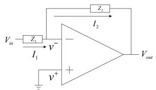
Figure 3. Circuit with impedances
