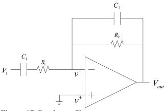
Figure 17. Band-pass filter
