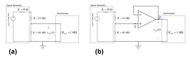
Figure 5. Comparison of circuit with and without buffer
